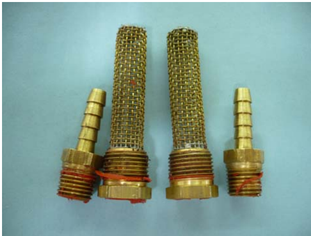
Picture 5 – finger strainer and outlet brass fitting disassembled
