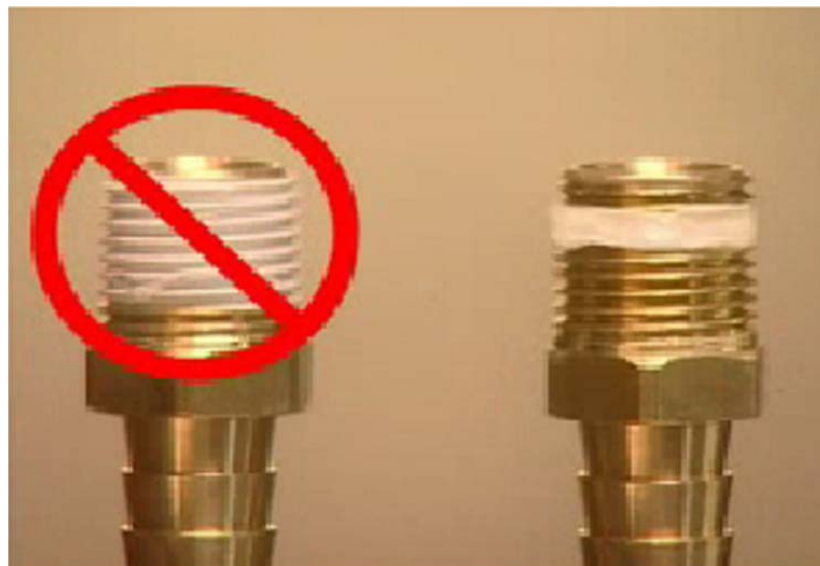
Picture 7 – proper application of sealant
